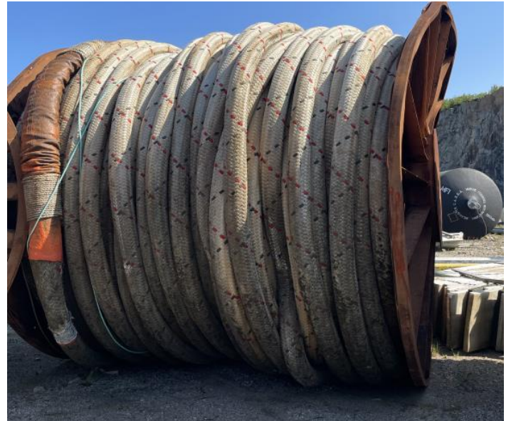
Fiber rope Dia 165 mm.
