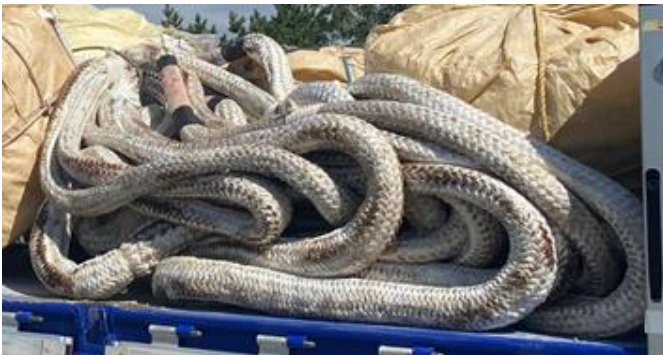
Dia 64 mm Endless Grommet Dyneema MBL 490 tons
