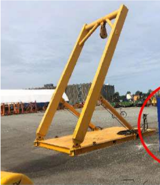
A-Frame 10 tonn Hydraulic sylinders, 210 Bar,
