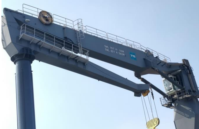
TTS Crane – 70 tons – CCLKO 2000-70-36,5
