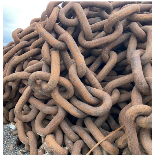
1800 meter studless chain dia 100 mm Grade R4. DNV Class.
