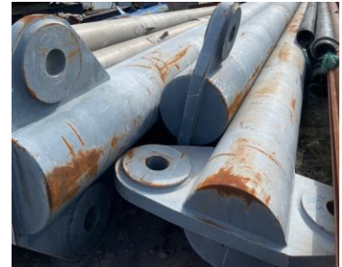
Item 166 Spread Beam WLL 380 tons. 9,7 and 11 m
