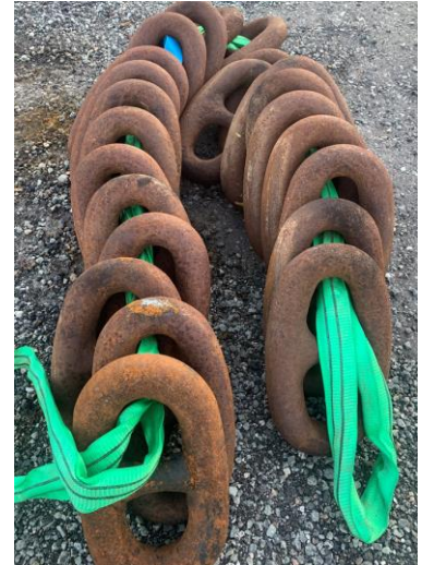
Ballast Links of chain
