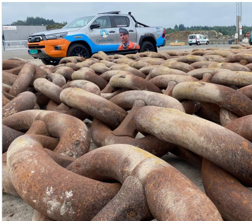
25,000 meter studlink and studless anchor-chain dia 120 mm, R4 DNV Class.
