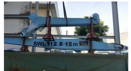
Item 306 Electro/Hydraulic Crane SWL 3 tons – 12 mtr radius
