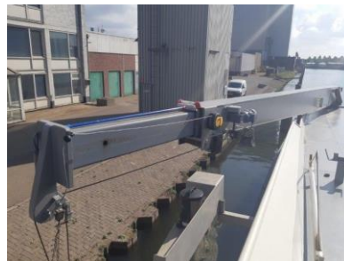
Item 5-15 Mistie Hose Crane 1500 kg at 18 mtr
