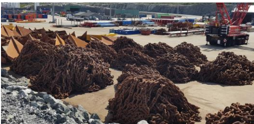
4500 meter anchor-chain dia 84 mm Grade R4, ABS Class.
