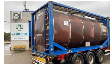
Item 202 ADR RID Tanks 24500 liters, 22 Bar, Stainless We several tanks in stock
