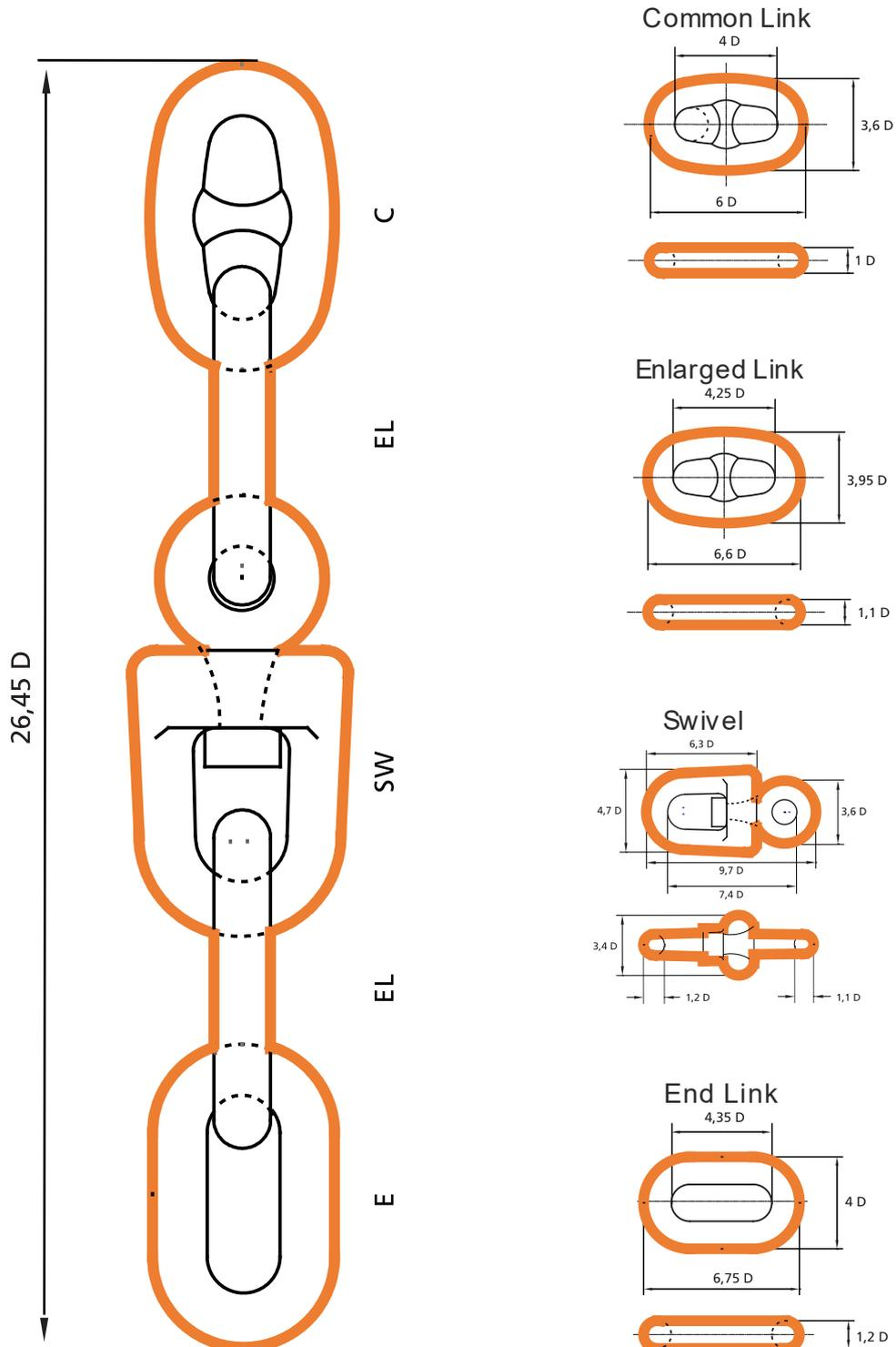
Weight unit is Kilograms. All measurements in mm. Measurements, weights, and drawings, are based on industry standards. Deviation margins need to be taken in mind, this is your own responsibility and not from Castle Hills AS.
