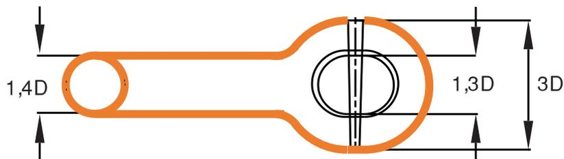
Weight unit is Kilograms. All measurements in mm. Measurements, weights, and drawings, are based on industry standards. Deviation margins need to be taken in mind, this is your own responsibility and not from Castle Hills AS.
